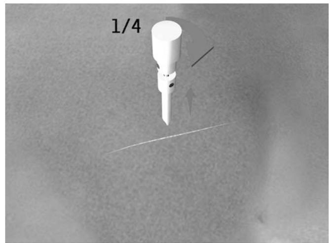
**Fig. 7** With a quarter of a turn the manipulator and the disconnecter are withdrawn
